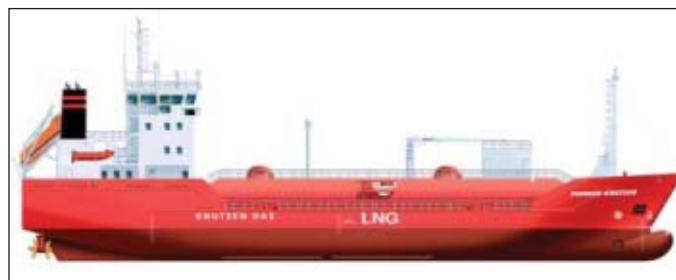
The 1,104-cu m LNG carrier Pioneer Knutsen, delivered in 2004, employs two engines for gas fuel only and two diesel engines in two separate engine rooms (Fig. 2).
