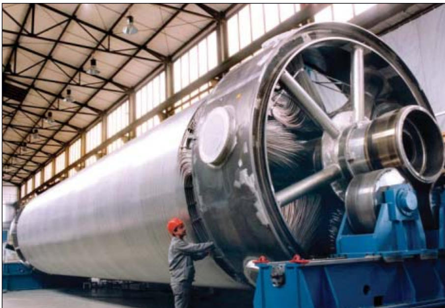
This is one of the spiral-wound heat exchangers manufactured by Linde for the Snøhvit project (Fig. 4; photo from Linde AG).
