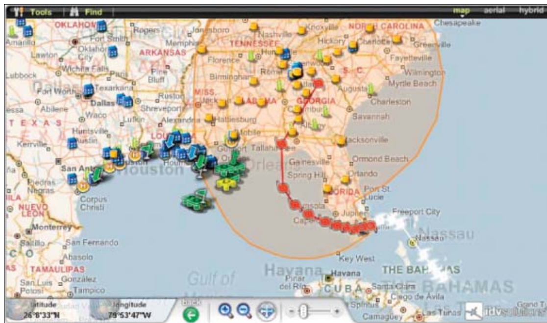
BP's hurricane monitoring system uses third-party web services to provide views of how real-time predictive hurricane paths relate to all of its facilities in the Gulf of Mexico (Fig. 1).
